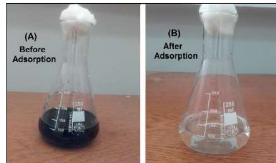
Figure 6: Shows 100 ml of 50 mg/l MG solution (a), treated solution (b).
